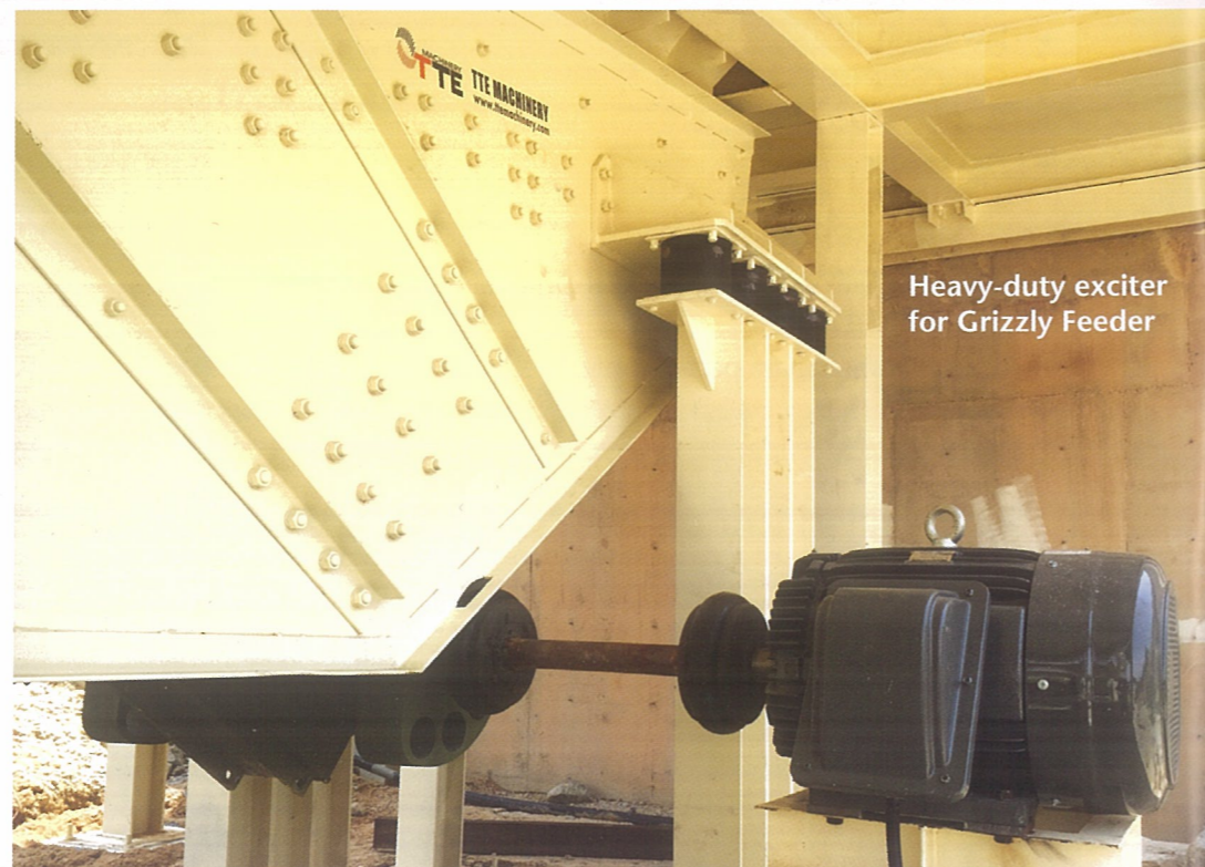
This Grizzly Feeder design can send material to Crusher evenly and continuously
