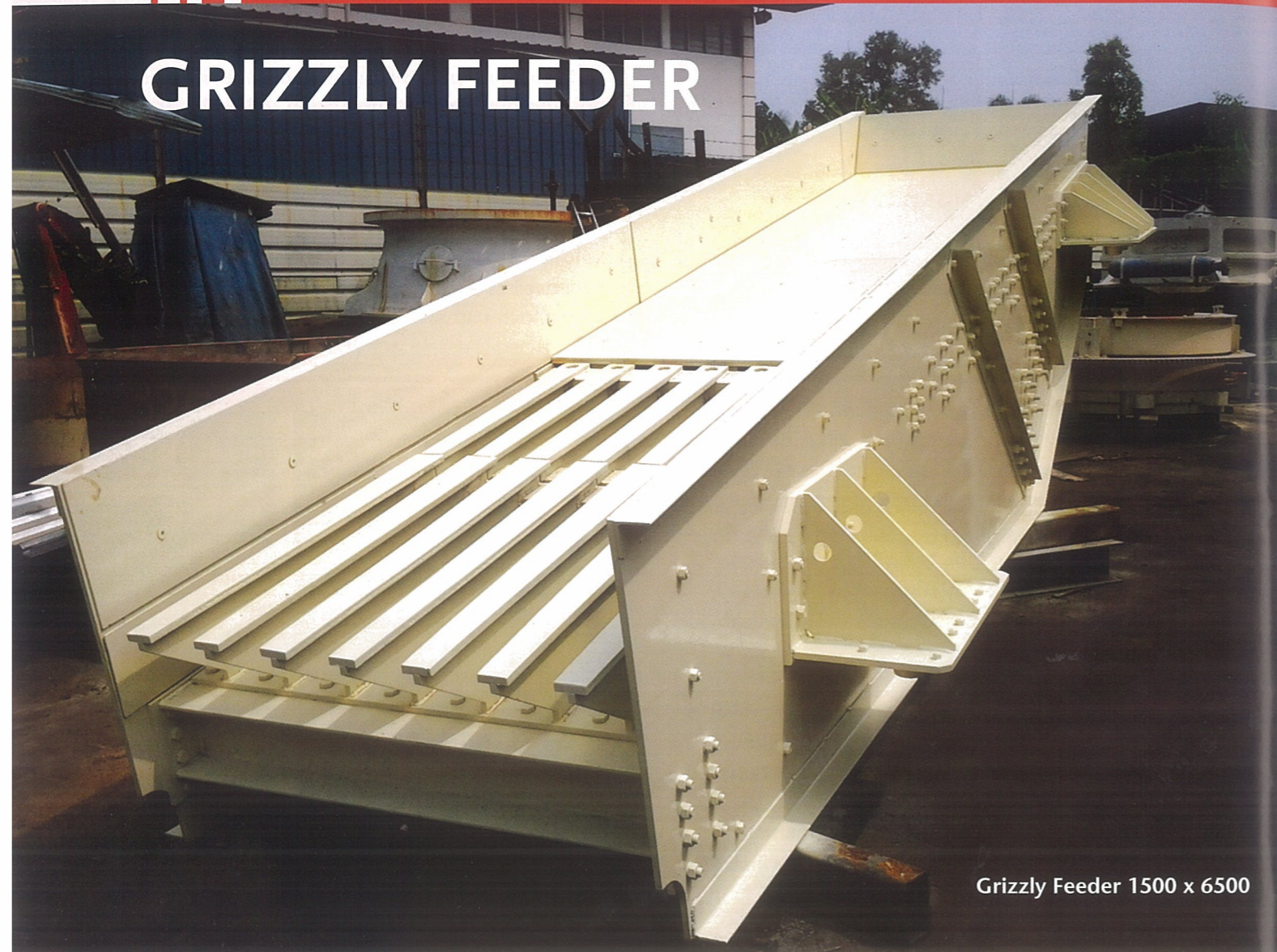
This Grizzly Feeder design can send material to Crusher evenly and continuously
